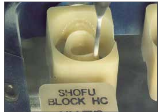
Shofu Blocks & Disks HC can be milled wet or dry in all standard milling units.
