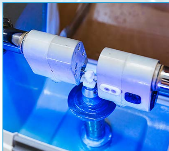
FIG 10. Milling the crown (HC Block, A3-LT; Shofu) with Cerec inLab MC XL (Dentsply Sirona).
