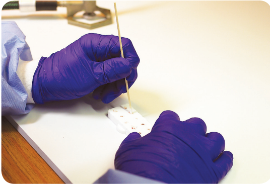
Figure 5. Collection of samples from BurButler block holes after autoclave cycle
